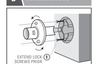
Align slots on escutcheon with screw holes. Align backplate & screw into ext. housing.
